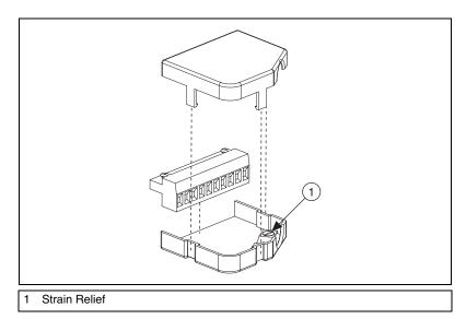
Figure 9. High Voltage Screw Terminal Backshell
